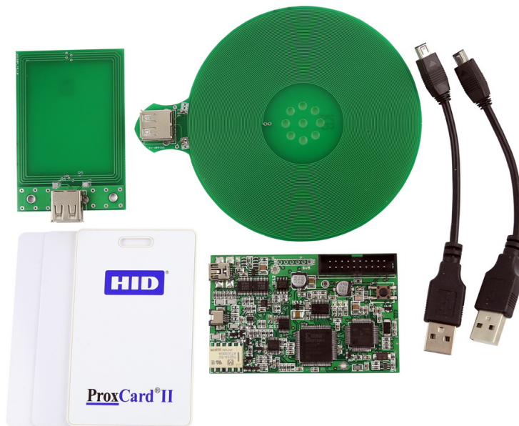
Figure 3: Proxmark III hardware kit. It also includes high- and low-frequency antennas, as well as examples of cards of different standards.
