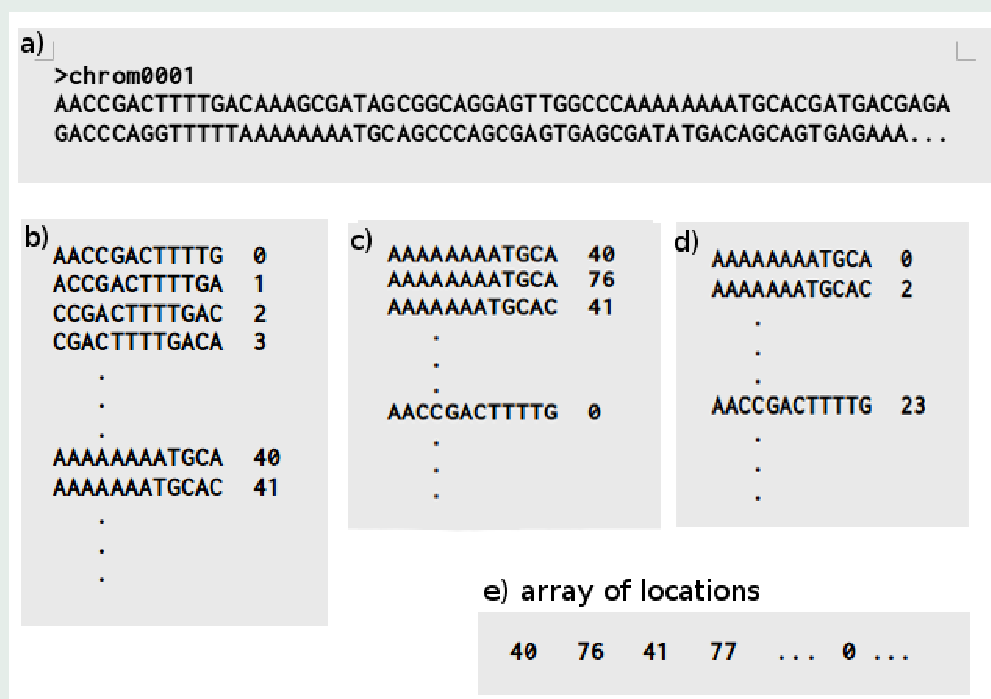
Figure 1: a) Genome sequence; b) All extracted n -mers; c) n -mers sorted with in-place radix sort; d) Only one copy of each n -mer and the pointer to the array of locations (e).
