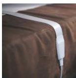
A thin piezo-electric force sensor placed under the mattress topper (from Beddit Ltd)
