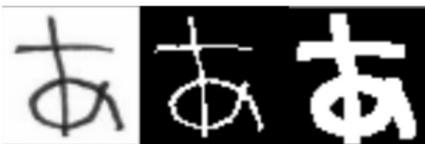
Figure 1. Left: initial image. Center: threshold image. Right: dilated image.
