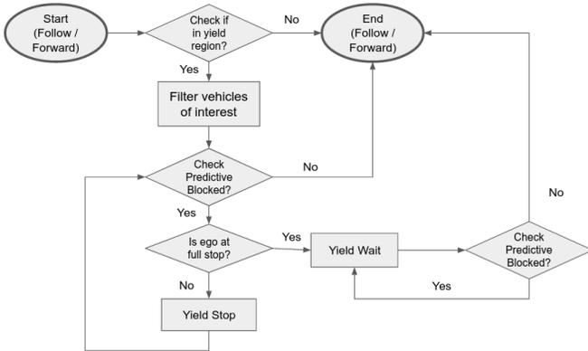
Fig. 4. Flow chart of yielding algorithm.
