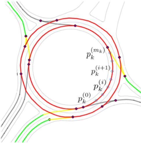
Fig. 2. Zones of a roundabout described by [3]. Here, green marked areas are decision zone, yellow marked areas are transition zone, red marked lanes are ring zone and gray marked lanes are exit zone
