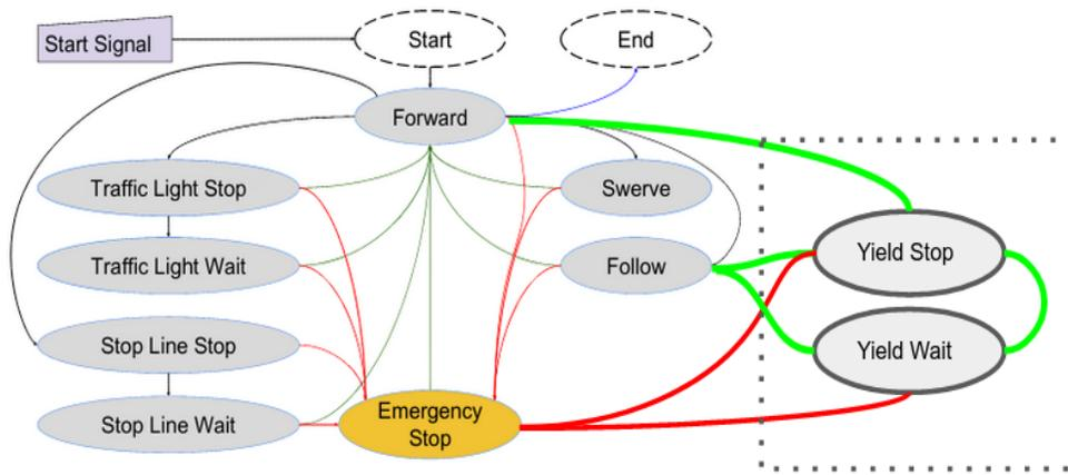
Fig. 3. Behaviour state machines of Open-planner [7]. Here, the newly implemented states are shown in dotted area.
