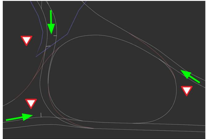
Fig. 5. An illustration of Autoware's vector map of Delta building roundabout we used for testing yielding scenarios. Here, green arrows show possible entry points with give-way sign on each entry
