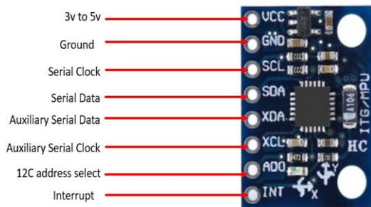
Fig. 5. An MPU6050 Pinout of MEMS MPU6050 module consisting of a 3-axis accelerometer and 3-axis gyroscope sensor
