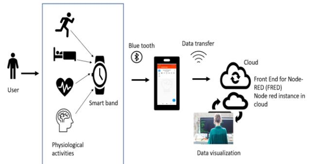
Fig. 7. Proposed real-time biofeedback system overview
