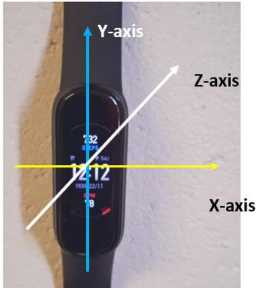
Fig. 1. Orthogonal planes on smart band depicting the X, Y, and Z-axis
