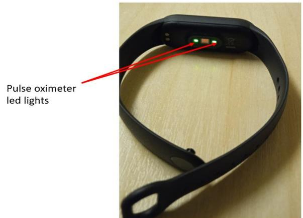
Fig. 2. Diagram indicating the location of Miband- five SpO<sub>2</sub> sensors, two led lights, and its capacitive proximity sensor.
