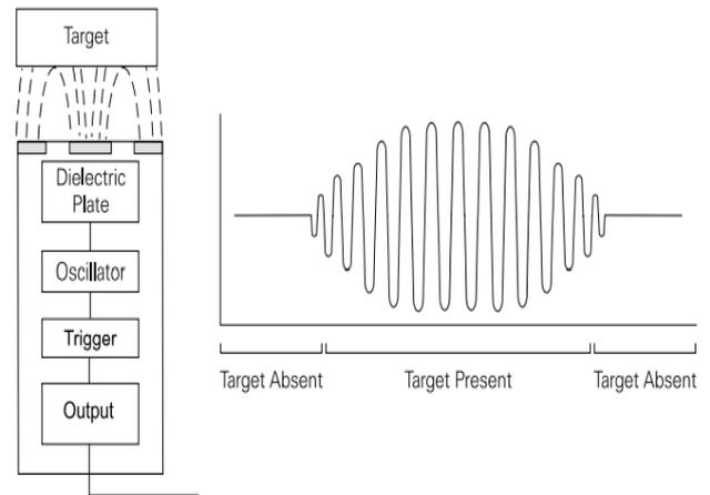
Fig. 3. Overview of the oscillatory circuit of the capacitive proximity sensor.
