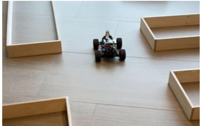
Figure 1. **Donkey Car Platform** – Track for autonomous driving scenario. The ego vehicle travels on the track avoiding collision with the walls and other stationary vehicles set on the track.
