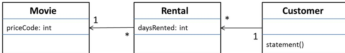
Figure 1. A class diagram of the starting point classes. Only the most important features are shown. The notation is UML
